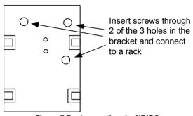
Figure 7 Rack mounting the XRICC
